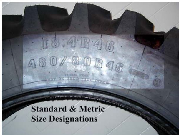
Figure 3. Standard and metric size designation.
