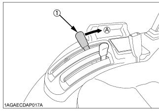
(1) Hydraulic control lever [Except B2320DTN, B2320HSDN] Position control lever [B2320DTN, B2320HSDN]
