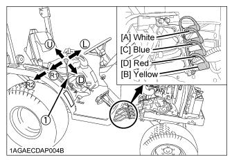
(1) Loader / Remote control valve lever
